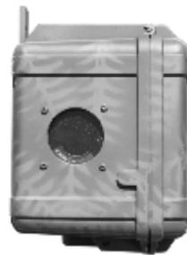
NORCAM uses quality single lens reflex digital cameras complete with a zoom lens that allows up to 6X magnification. The units are designed to be used in remote areas where there is no external power.
